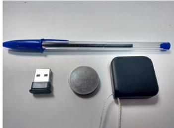
Fig. 1. The BLE advertiser (right), receiver (left), and a power cell CR2450, that is inside the advertiser (center). The pen is shown to compare the sizes.
